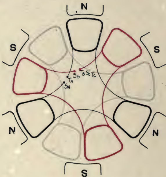
FIG. 233.—Six-pole, Three-phase, Short-coil Winding.
